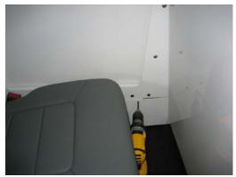
Attach to K9 housing using #10 x <sup>3</sup>/<sub>4</sub>" sheet metal screws.
